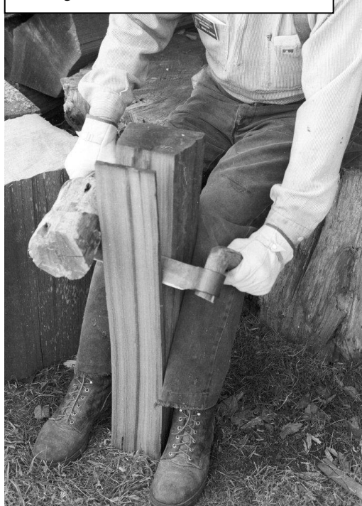
Making redwood shakes with froe & mallet
